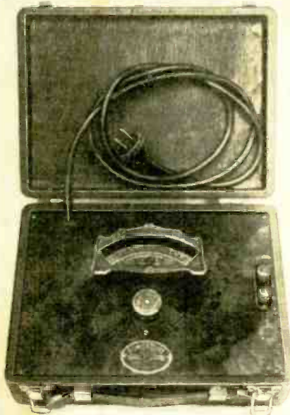
A portable test oscillator which has many uses. (No. 101)
