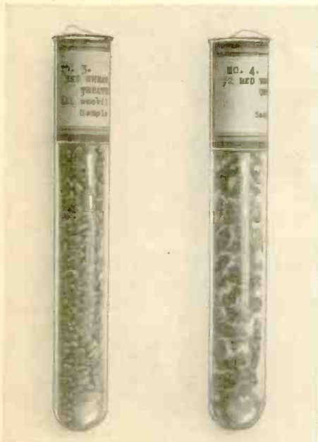
Tube at left shows weevil-infested wheat, treated by Mr. Davis' system for six seconds, the weevils being exterminated. Tube at right contains wheat from same lot, but untreated—wheat destroyed.
