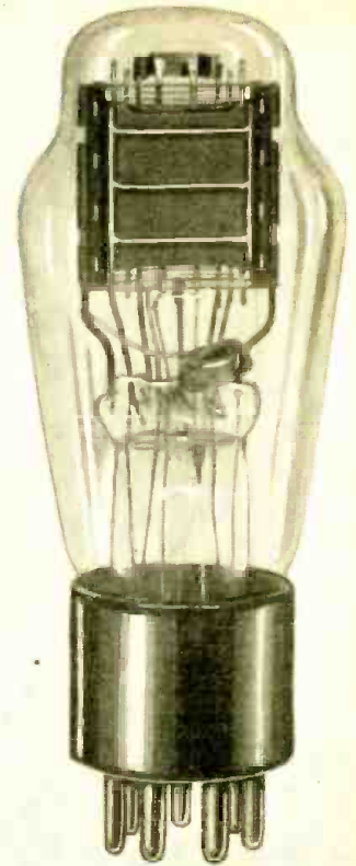
Appearance of the new 59 power amplifier tube of the triple-grid type. Several ways of operating this tube are discussed by the author in the present article.
